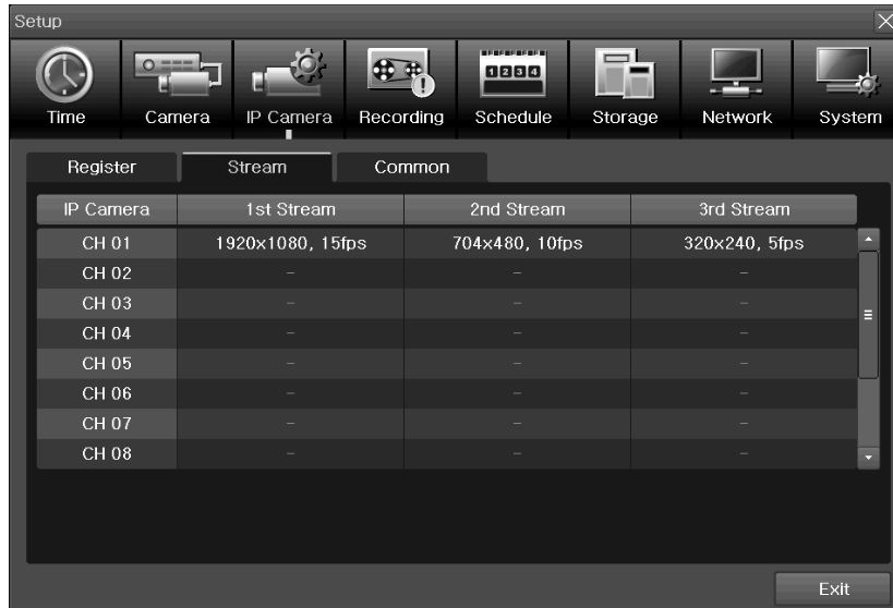
[Figure 3-19. IP Camera Stream Setup]
