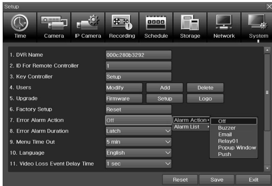
[Figure 3-48. Alarm Action]
